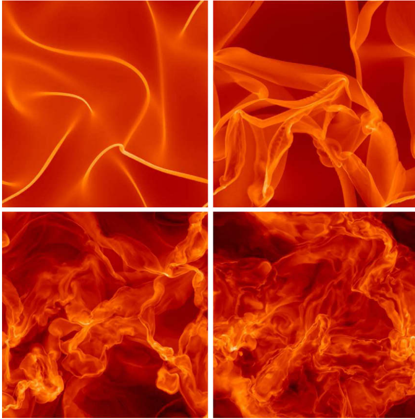
Fig. 17. Supersonic turbulence simulation with PPML on a 512^3 grid. Four snapshots show the density field on a slice x \equiv 0 illustrating a transition to fully developed turbulence with M_s \approx M_A \approx 10 . The transition includes formation of first strong shocks on the caustics of the initial solenoidal velocity field ( t = 0.5t_d , top-left), shock interactions and active development of first shear instabilities ( t = 1t_d , top-right), and a gradual transition to a statistical steady state ( t = 2t_d and 4t_d , bottom row). The standard logarithmic black–red–white color ramp shows high-density regions in light-red and rarefactions in black. (For interpretation of the references to colour in this figure legend, the reader is referred to the web version of this article.)
